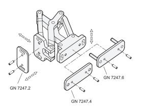
The multiple-joint hinges can be adjusted in three planes during installation. For example, this allows adjustment for tolerances or establishing of required compressive forces for seals.
