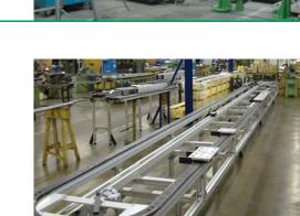
HepcoMotion® **PRT2 / DLS** HepcoMotion Ring & Track (PRT2) and (DLS) Driven Actuator system under test in our Tiverton factory.
