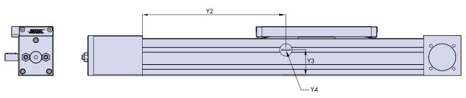
Re-lubrication of the ball guide carriage block is via an access point in the side of the beam (see above), which is closed off with a threaded plug. The lubrication interval depends on the length of stroke, speed and duty. For further details regarding lubrication procedures please contact Hepco's technical department.
