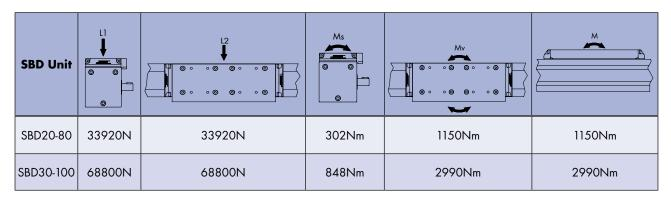
The table below includes the parameters necessary to calculate the performance and duty of an SBD system.
