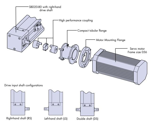
The hollow shafted arrangement may offer a more compact and lower cost means of retro-fitting a motor and/or gearbox onto an SBD. For further details of motor connections please visit <a href="www.HepcoMotion.com/sbddatauk">www.HepcoMotion.com/sbddatauk</a> and select datasheet No. 1 SBD motor connections.
